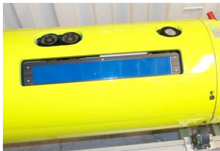
IBMT 3-frequency side scanner alone and integrated in AUV (pressure balanced electronic is integrated in the transducer housing).
