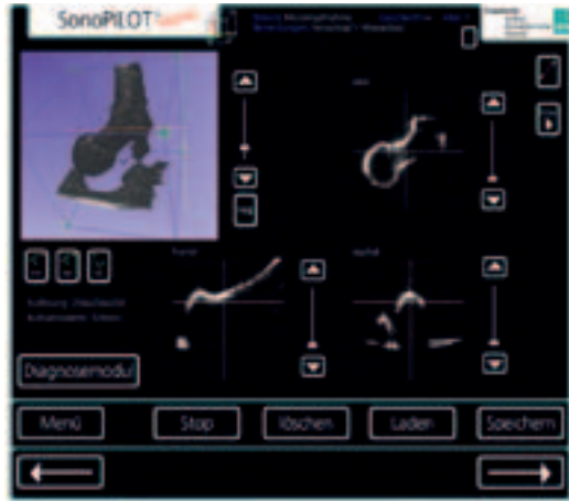
Left: Prototype of the "SonoPilot@ortho". Right: 3-D reconstruction of a femur with merged, automatically detected position and size of the femur head. The automatic detection of anatomical landmarks provides a basis for using imaging in navigation systems.
