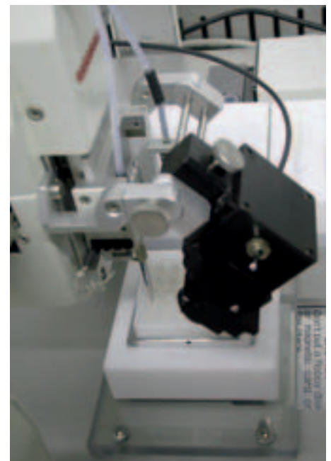
Nanoplotter (GeSIM mbH) during loading of a cryosubstrate with a capacity of 30 x 25 µl. The addition of cryoprotectives such as glycerol or DMSO can be precisely controlled in the picoliter range.
